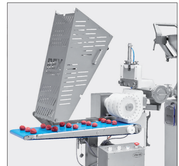
High performance thanks to multi-row form rollers
