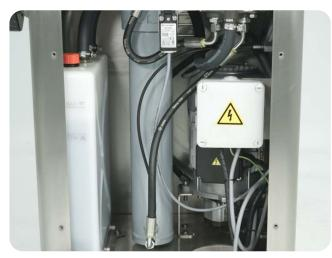
Powerful hydraulic system. Transparent oil reservoir, completely independent.
